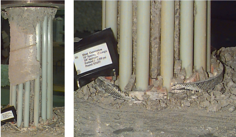
FIGURE 45 PHOTOGRAPHS OF COLUMN O, SHOWING END CIRC FAILURE BEFORE BUCKLING OF LONGIS
