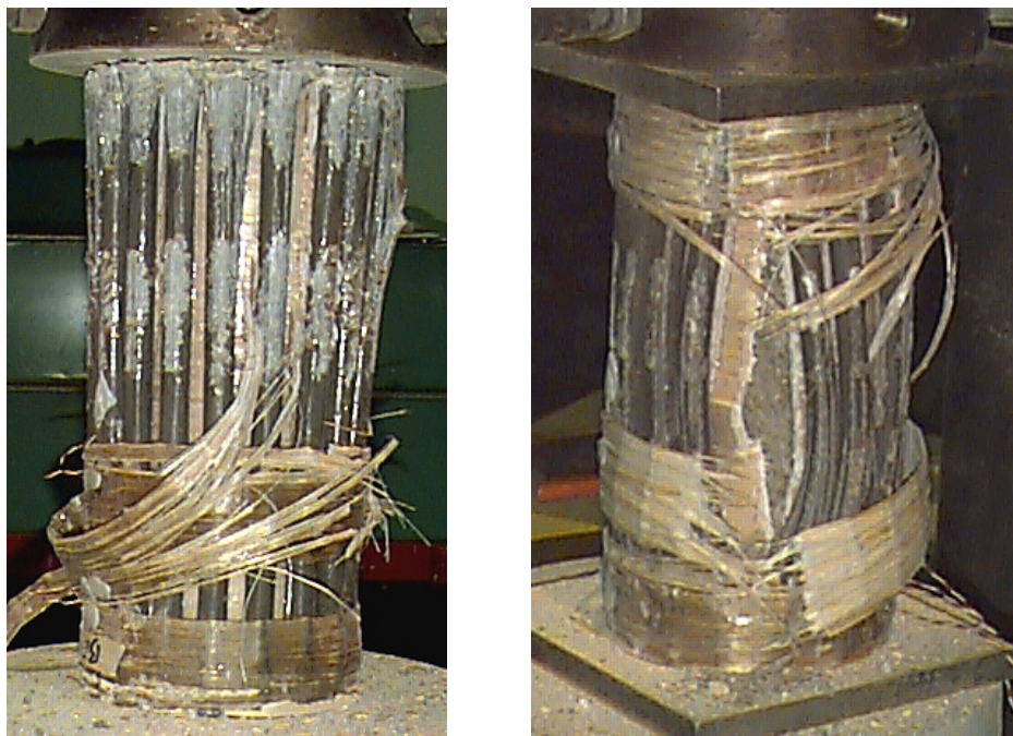
FIGURE 54 COLUMN B IN AXIAL COMPRESSION, SHOWING FAILURE OF 4" END WRAPS
