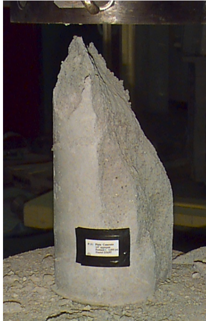
FIGURE 25 PHOTOGRAPH OF CONTROL SPECIMEN AFTER FAILURE
