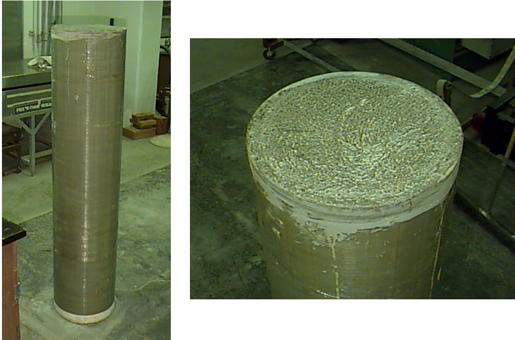
FIGURE 64 PHOTOGRAPHS OF 4 TH GENERATION COLUMN FILLED WITH HIGH STRENGTH CONCRETE
