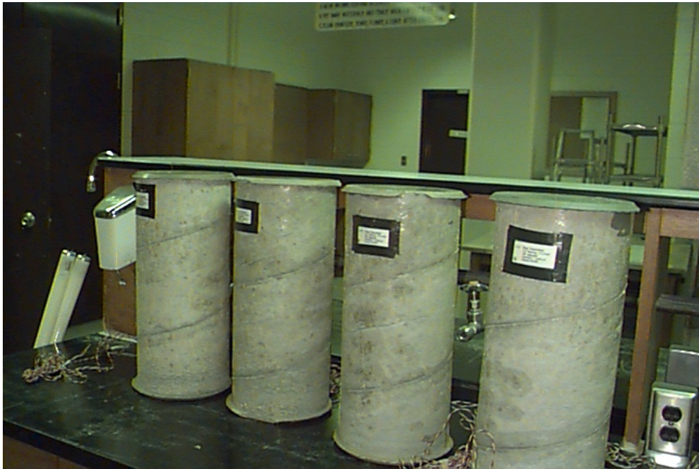
FIGURE 19 PHOTOGRAPH OF 1 ST GENERATION COLUMNS WITH SULFUR ENDCAPS
