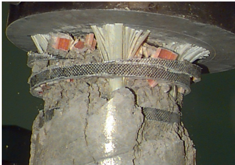
FIGURE 26 PHOTOGRAPH OF TYPICAL END FAILURE FOR 1 ST GENERATION COLUMN
