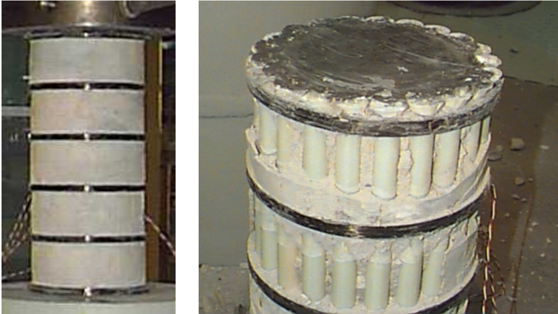
FIGURE 49 PHOTOGRAPHS OF COLUMN G IN AXIAL COMPRESSION, END FAILURE SHOWN
