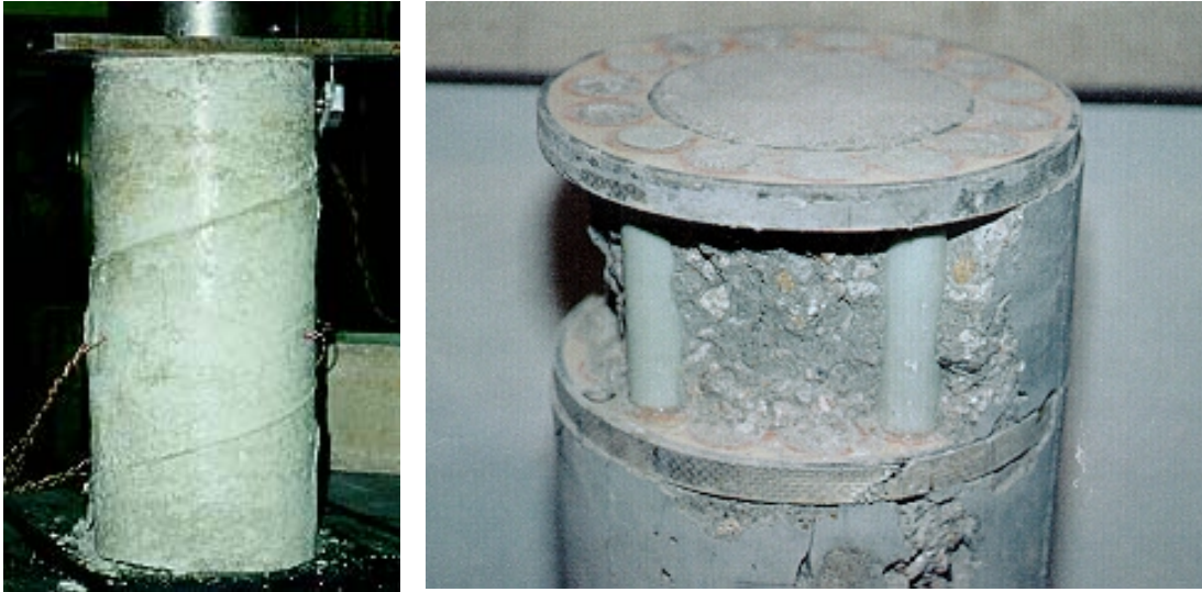
FIGURE 41 PRELIMINARY TEST AND END FAILURE FOR CONFIGURATION WITH 6 CIRCS, 5 LONGIS
