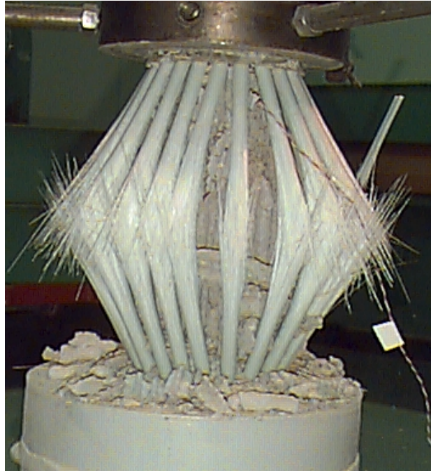
FIGURE 52 PHOTOGRAPH OF COLUMN J IN AXIAL COMPRESSION, BUCKLING OF THE LONGS
