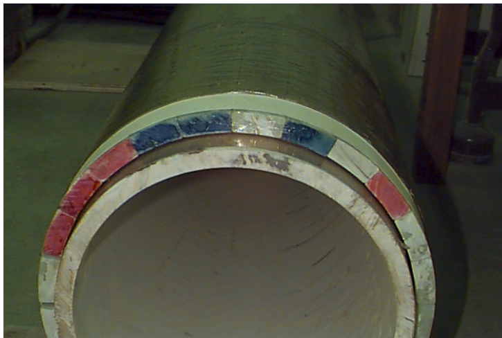
FIGURE 63 PHOTOGRAPH OF FAN-SHAPED LONGIS ON MANDREL
