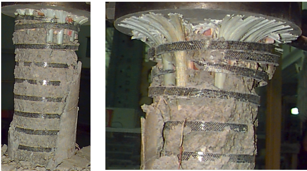
FIGURE 43 PHOTOGRAPHS OF COLUMN B IN AXIAL COMPRESSION, SHOWING BROOMING OF THE LONGIS
