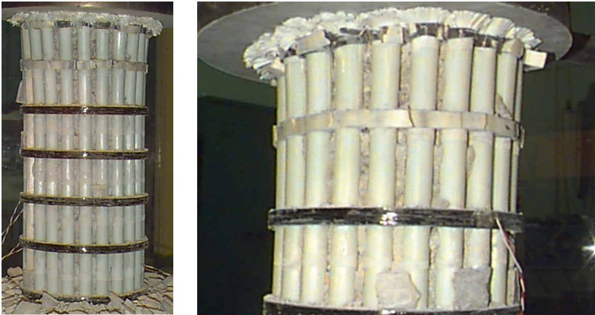
FIGURE 50 PHOTOGRAPHS OF COLUMN H IN AXIAL COMPRESSION, BROOMING OF LONGIS SHOWN
