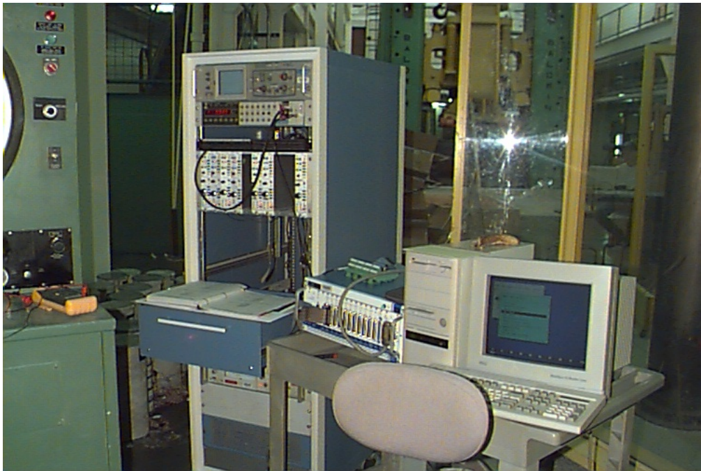
FIGURE 23 PHOTOGRAPH OF MEGADECK® DATA ACQUISITION SYSTEM
